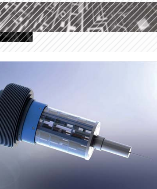
Figure 1. Main components and architecture of the robotic system. An actuation system transmits motion to the flexible tip through an array of concentric cylinders (like pistons). This way, the actuation system is decoupled from the tip, and enables changing the tip during surgery.
