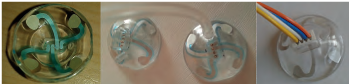
Figure 2. The contact lens 20 mm-diameter rigid scleral lens is connected to four 3 mm electrodes, which are in turn directly connected to the electrostimulating device.
