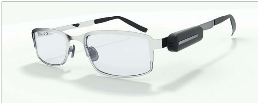
Figure 1. The Visual Behavior Monitor (Vivior AG, Zürich, Switzerland); a small device with distance, ambient light and orientation and motion sensors that clips onto a pair of spectacles.
